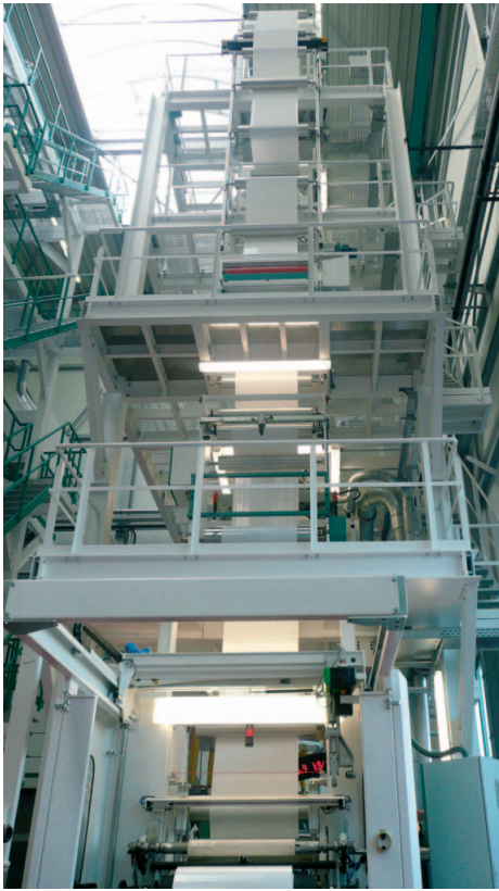
For the first time, KUHNE will present a three-layer coextrusion blown film line for the production of FFS film in live operation at Plast 2009
