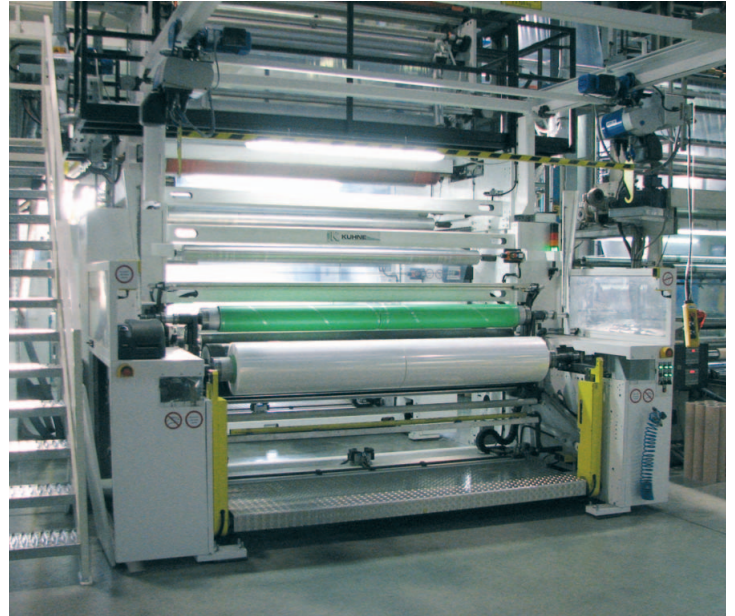
KUHNE's three-layer blown film line meets Idealplast's specifications right down to the double station winder
