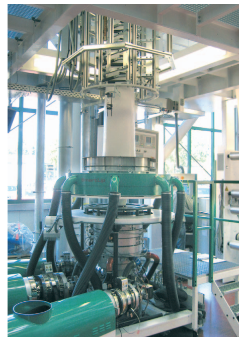
Equipped with the twice-improved Smart Lip Maximizer high-performance cooling ring, the FFS line achieves an outstanding throughput rate of 360 kg/h
